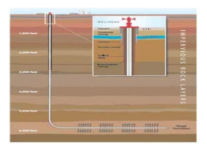
The Shale gas well is typically 5,000 to 8,000 feet down below the earth's surface. After a well is drilled and secured, a chemical mixture, made up of 98% sand and water along with a small amount of chemical additives, is injected at a very high pressure to fracture the shale. The sand keeps the fracture open and serves as a conduit for extracting the natural gas.
